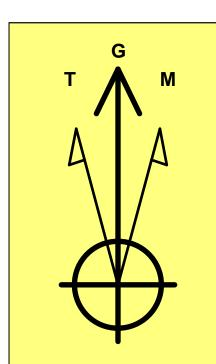
**Azimuths to Grid North** True North: -0.24° Magnetic North: 6.48°
