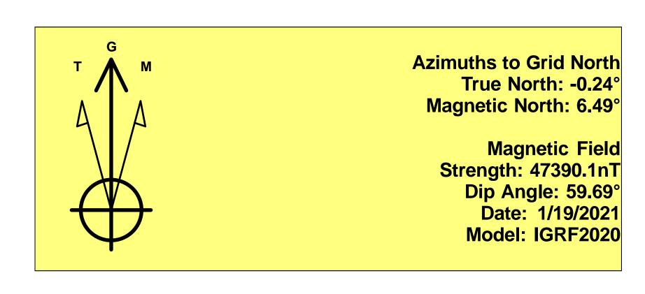
To convert a Magnetic Direction to a Grid Direction, Add 6.49° To convert a Magnetic Direction to a True Direction, Add 6.72° East To convert a True Direction to a Grid Direction, Subtract 0.24°
