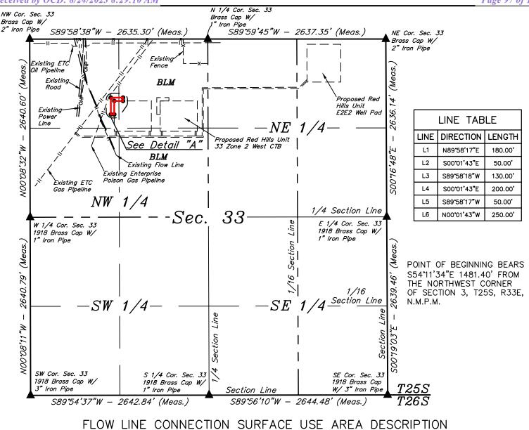
BEGINNING AT A POINT IN THE NW 1/4 NW 1/4 OF SECTION 33, T25S, R33E, N.M.P.M., WHICH BEARS S54\*11'34"E 1481.40' FROM THE NORTHWEST CORNER OF SAID SECTION 33, THENCE N89\*58'17"E 180.00'; THENCE S00\*01'43"E 50.00'; THENCE S89\*58'18"W 130.00'; THENCE S00\*01'43"E 200.00'; THENCE S89\*58'17"W 50.00'; THENCE N00\*01'43"W 250.00' TO THE POINT OF BEGINNING. CONTAINS 0.436 ACRES MORE OR LESS.
