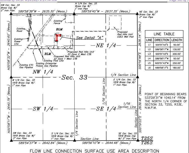
BEGINNING AT A POINT IN THE NE 1/4 NW 1/4 OF SECTION 33, T25S, R33E, N.M.P.M., WHICH BEARS S33°29'31"W 1040.14' FROM THE NORTH 1/4 CORNER OF SAID SECTION 33, THENCE S00°01'43"E 50.00'; THENCE S89°58'17"W 130.00'; THENCE S00°01'43"E 200.00'; THENCE S89°58'17"W 50.00'; THENCE N00°01'43"W 250.00'; THENCE N89°58'17"E 180.00' TO THE POINT OF BEGINNING. CONTAINS 0.436 ACRES MORE OR LESS.
