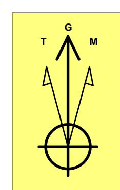
Azimuths to Grid North True North: -0.40° Magnetic North: 6.23°
