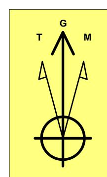
Azimuths to Grid North True North: -0.40° Magnetic North: 6.24°
