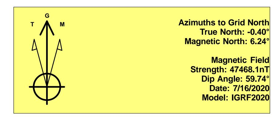
To convert a Magnetic Direction to a Grid Direction, Add 6.24° To convert a Magnetic Direction to a True Direction, Add 6.64° East To convert a True Direction to a Grid Direction, Subtract 0.40°
