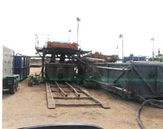
Above: Centrifugal Closed Loop System
