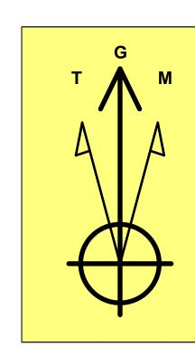
**Azimuths to Grid North** True North: -0.40° Magnetic North: 6.02°
