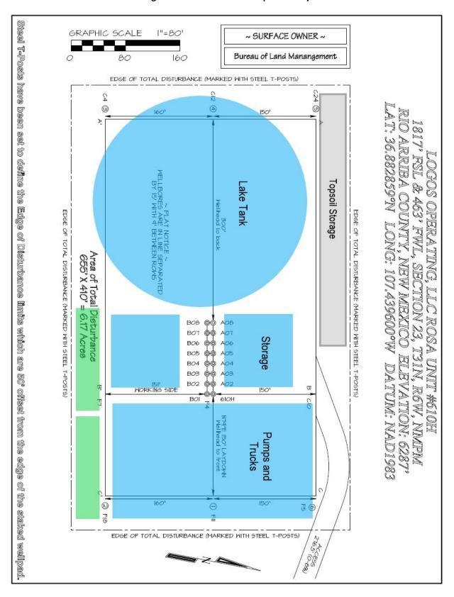
Figure 11. Rosa Pad 10 Completion Layout
