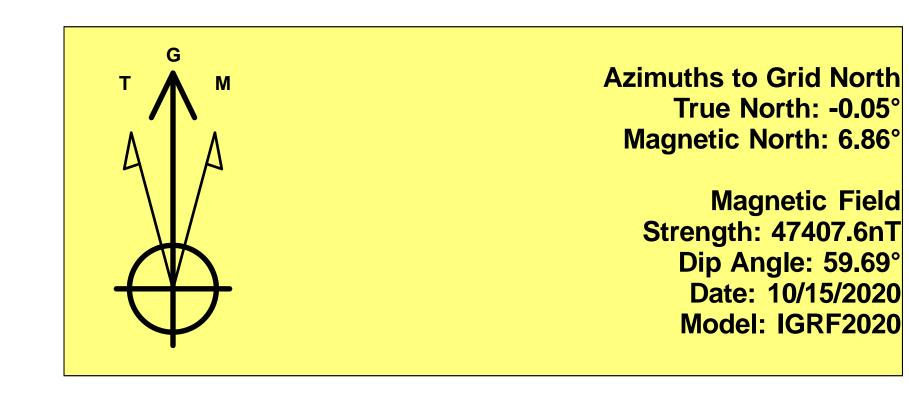
To convert a Magnetic Direction to a Grid Direction, Add 6.86° To convert a Magnetic Direction to a True Direction, Add 6.92° East To convert a True Direction to a Grid Direction, Subtract 0.05°
