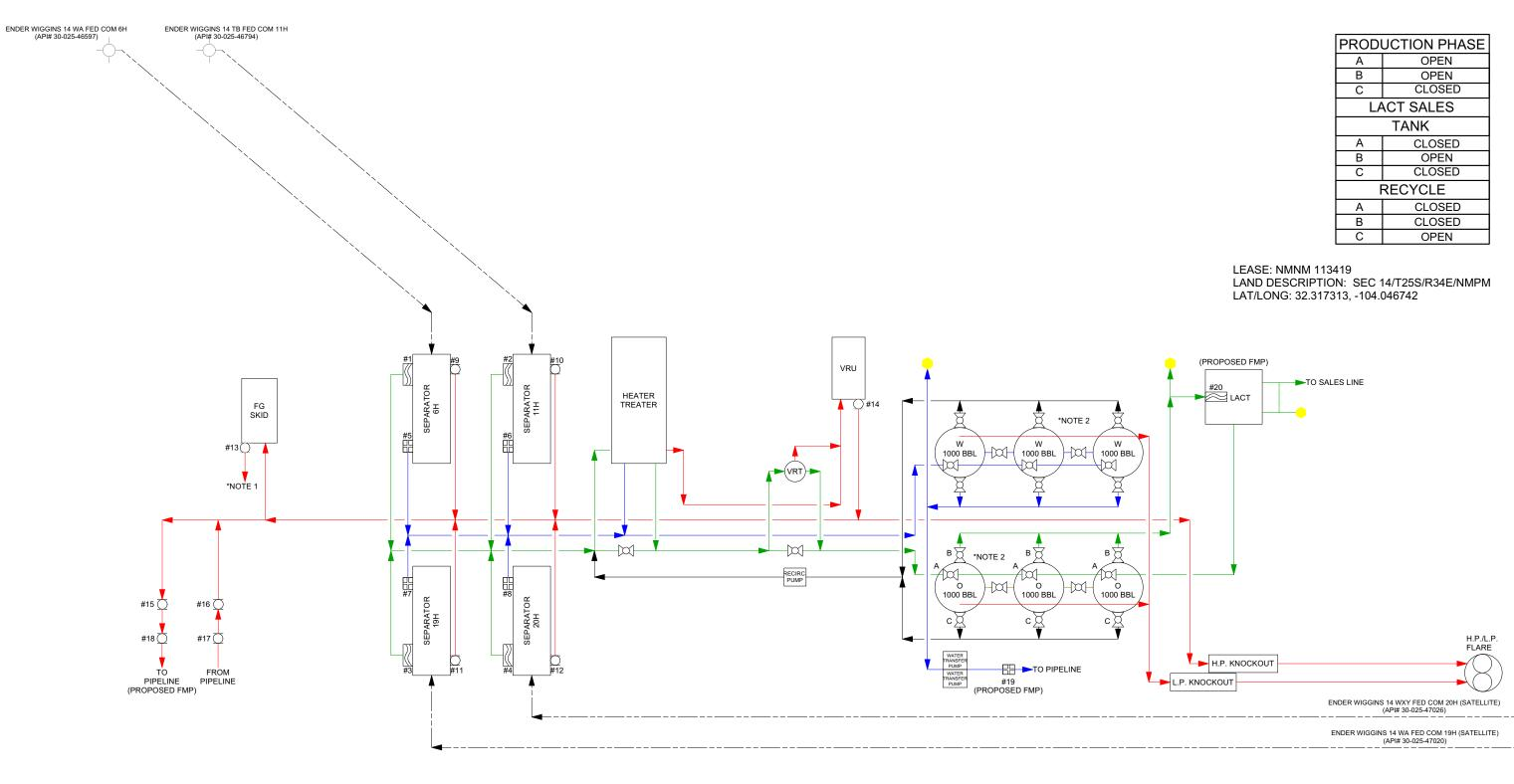
1. FUEL GAS IS ROUTED THROUGHOUT THE FACILITY 2. PROCESS FLOW IS CAPTURED IN VALVE POSITIONING TABLE.
