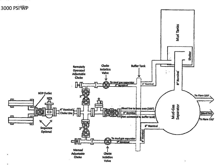
Variance request: A variance is requested to use a Multi Bowl System and Flex Hose as the choke line from the BOP to the Choke Manifold. If this hose is used, a copy of the manufacturer's certification and pressure test will be kept on the rig.
