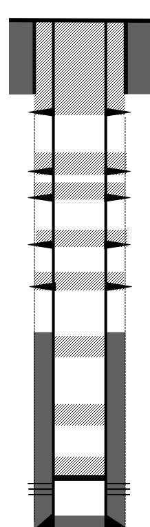
8-5/8" J-55 24# casing @ 269'. Cemented with 130 sks Class B. Circulated cement to surface. Hole size: 12-1/4
