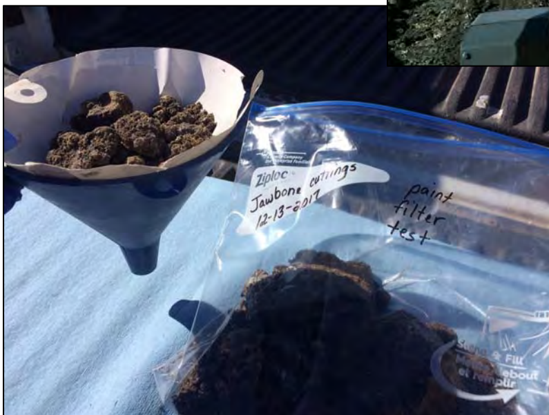
Paint filter test of mixed cuttings 12/13/2017
