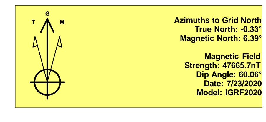
To convert a Magnetic Direction to a Grid Direction, Add 6.39° To convert a Magnetic Direction to a True Direction, Add 6.73° East To convert a True Direction to a Grid Direction, Subtract 0.33°
