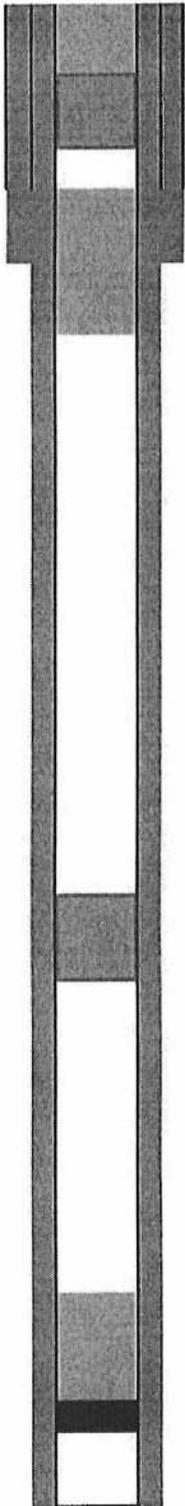
**Surface plug: 574' to surface. 60sx.** INSTALL DRY HOLE MARKER
