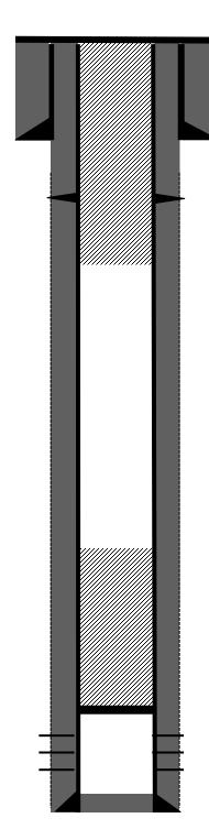
7" 20# casing @ 128'. Cemented with 65 sks Class B cement. Hole size: 9-1/4". Circulate 3 bbls cement to surface.
