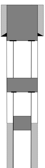
Plug 4 (Surf Shoe) – perf @ 180' attempt to establish circulation, Pump/circ. Cmt to surf w/~94 sx if no circ., ~8 sx need to cap inside casing KB = 13 ft GL = 6,583 ft API# 30-039-20936
