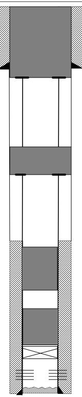
Plug 4 (Surf Shoe) – perf @ 180' attempt to establish circulation, Pump/circ. Cmt to surf w/~70 sx if no circ., ~8 sx need to cap inside casing KB = 13 ft GL = 6,583 ft API# 30-039-20936
