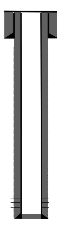
8-5/8" 24# casing @ 129'. Cemented with 85 sks Class B cement. Hole size: 12-1/4". Circulate 7 bbls cement to surface.
