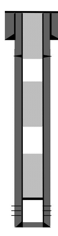
8-5/8" 24# casing @ 129'. Cemented with 85 sks Class B cement. Hole size: 12-1/4". Circulate 7 bbls cement to surface.
