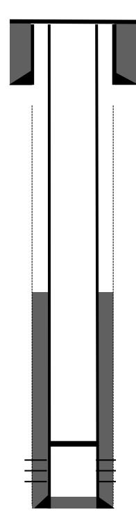
$7"\,20\#$  casing @ 139'. Cemented with 65 sks Type 5 cement. Hole size: 8-3/4". Circulate 6 bbls cement to surface.
