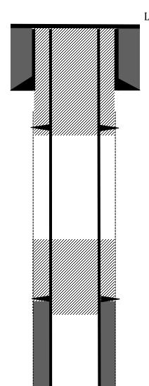
$7^{\prime\prime}$  20# casing @ 139'. Cemented with 65 sks Type 5 cement. Hole size: 8-3/4". Circulate 6 bbls cement to surface.
