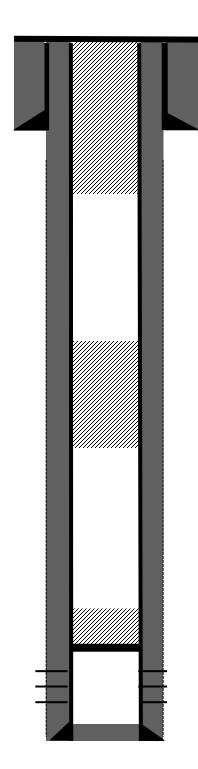
$7^{\prime\prime}$  20# casing @ 132'. Cemented with 65 sks Type 5 cement. Hole size: 8-3/4". Circulate 5 bbls cement to surface.
