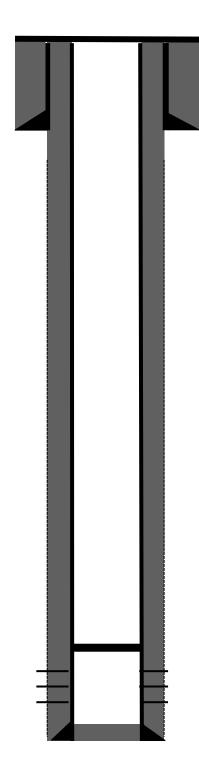
7" 20# casing @ 132'. Cemented with 65 sks Type 5 cement. Hole size: 8-3/4". Circulate 5 bbls cement to surface.
