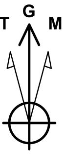
**Azimuths to Grid North** True North: -0.44° Magnetic North: 5.82°
