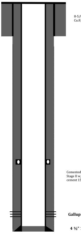
8-5/8'' J-55 24# casing @ 210'. Cemented with 135 sks Class B (159 Cu.ft). Circulated 1.5 bbls cement to surface. Hole size: 12-1/4
