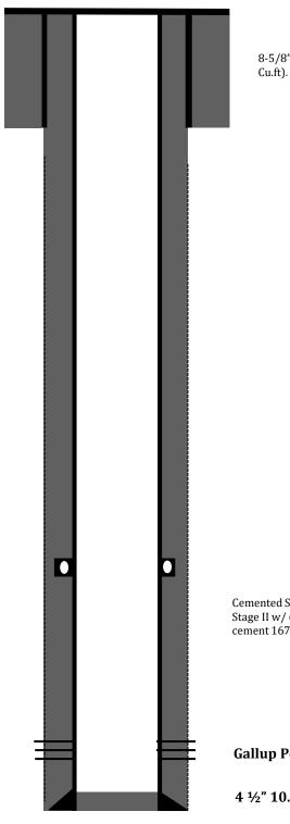
$8{\text{-}}5/8"$  J-55 24# casing @ 220'. Cemented with 135 sks Class B (159 Cu.ft). Circulated 5 bbls cement to surface. Hole size:  $12{\text{-}}1/4$
