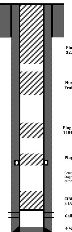
8-5/8" J-55 24# casing @ 220'. Cemented with 135 sks Class B (159 Cu.ft). Circulated 5 bbls cement to surface. Hole size: 12-1/4
