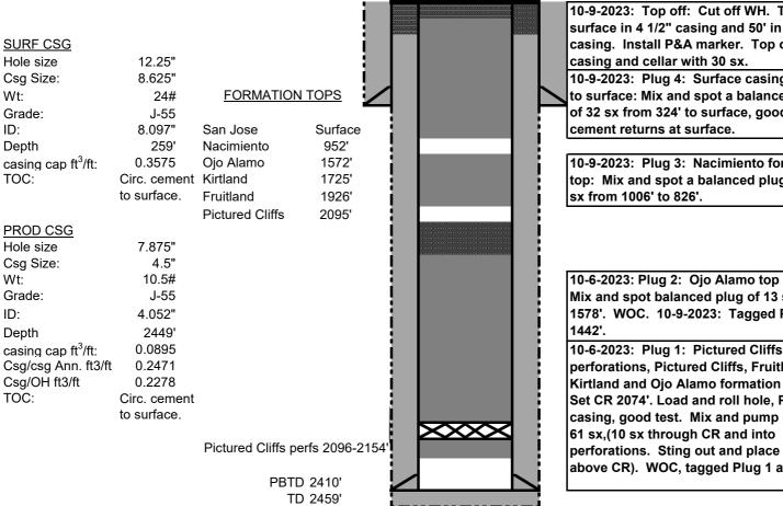
10-9-2023: Top off: Cut off WH. TOC at surface in 4 1/2" casing and 50' in 8 5/8" casing. Install P&A marker. Top off casing and cellar with 30 sx.
