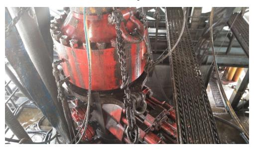
Figure 1: Winch System attached to BOP Stack
