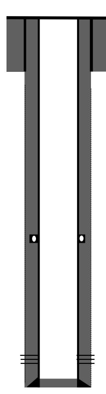
8-5/8" J-55 24# casing @ 230'. Cemented with 135 sks Class B (159 Cu.ft). Circulated 4 bbls cement to surface. Hole size: 12-1/4
