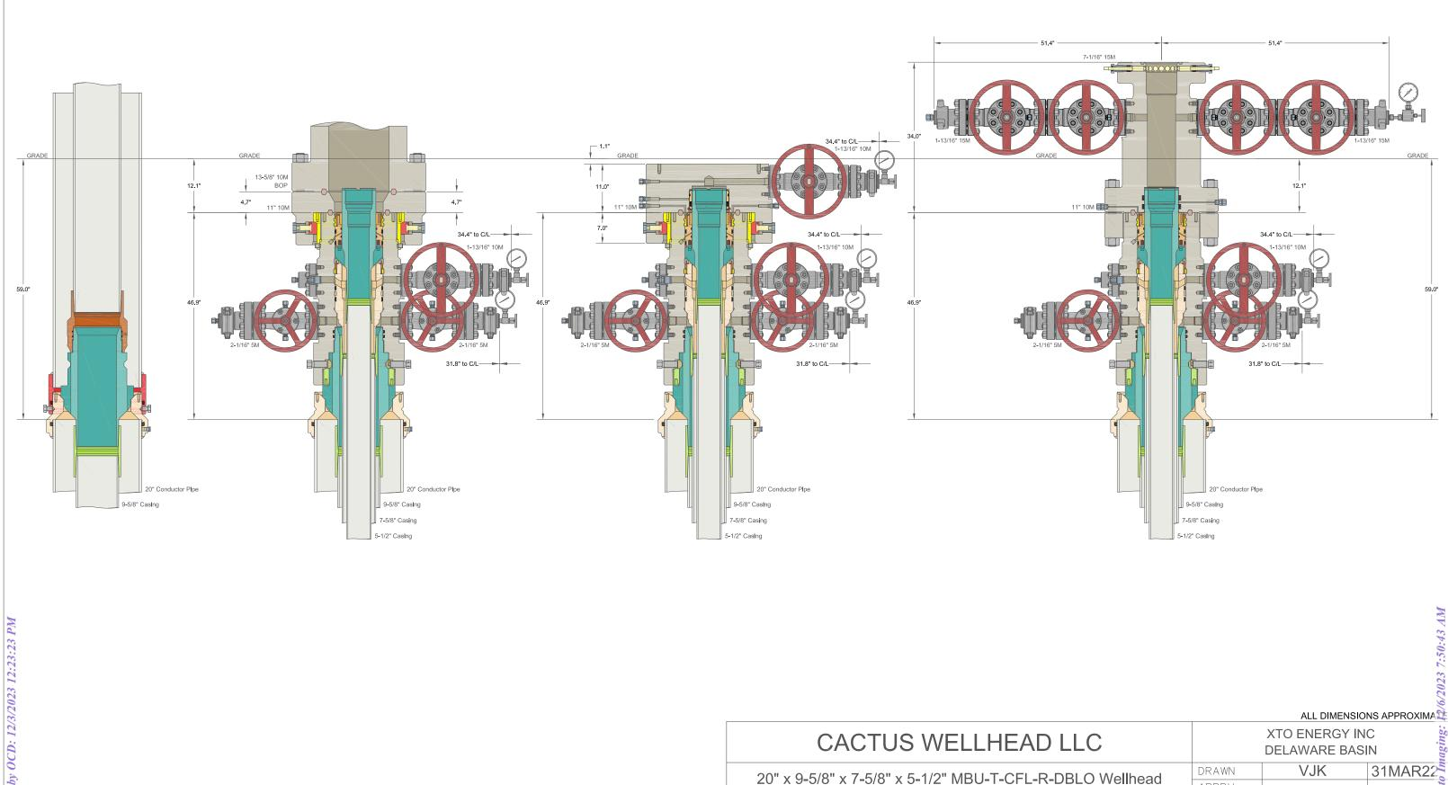
20" x 9-5/8" x 7-5/8" x 5-1/2" MBU-T-CFL-R-DE With 11" 10M x 7-1/16" 15M CTH-DBLHPS T And 9-5/8", 7-5/8" & 5-1/2" Pin Bottom Mandrel C
