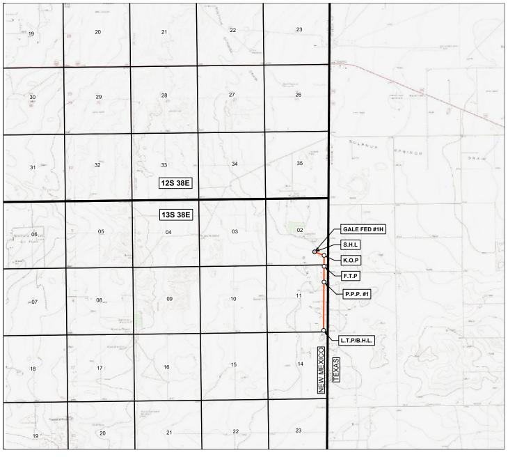
LEASE NAME AND WELL NUMBER: <u>GALE FED #1H</u> LATITUDE: <u>N 33.216290</u> LONGITUDE: <u>W 103.063779</u> ELEVATION:  $\underline{3804}$ ' DESCRIPTION:  $\underline{1068}$ ' FSL &  $\underline{1086}$ ' FEL
