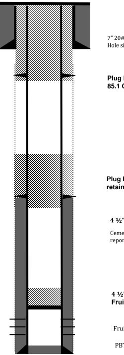
7" 20# casing @ 139'. Cemented with 65 sks Type 5 cement. Hole size: 8-3/4". Circulate 6 bbls cement to surface.
