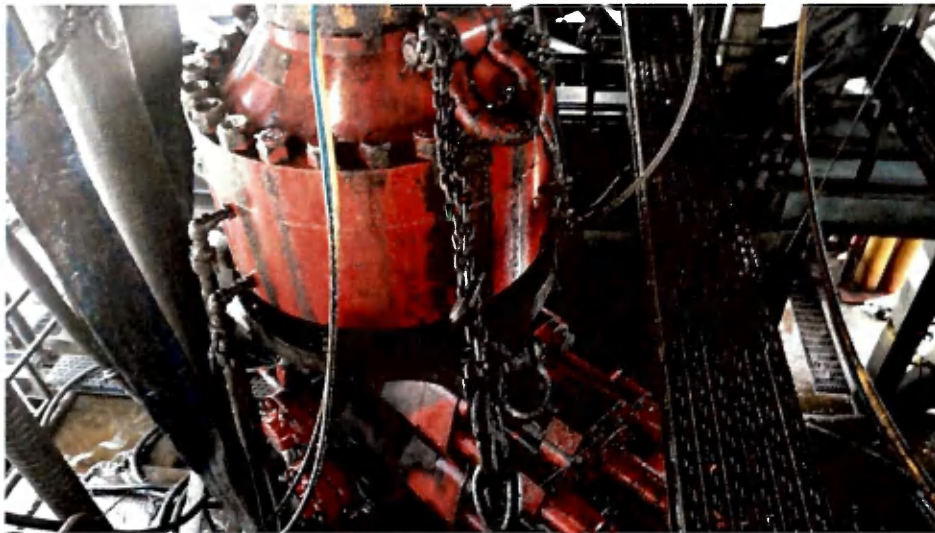
Figure 1: Winch System attached to BOP Stack
