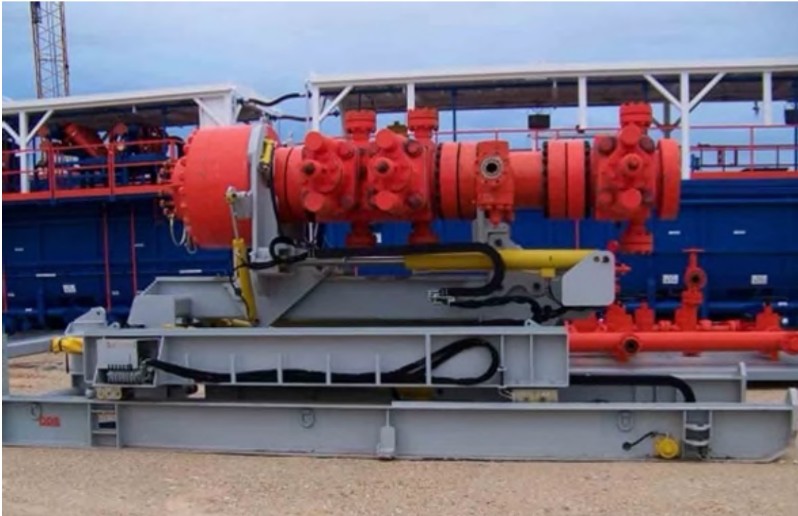
Figure 4. BOP handling system
