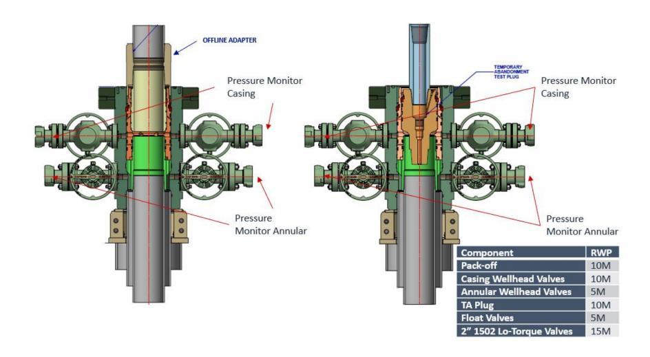
Figure 2: Cactus TA Plug and Offline Adapter Schematic
