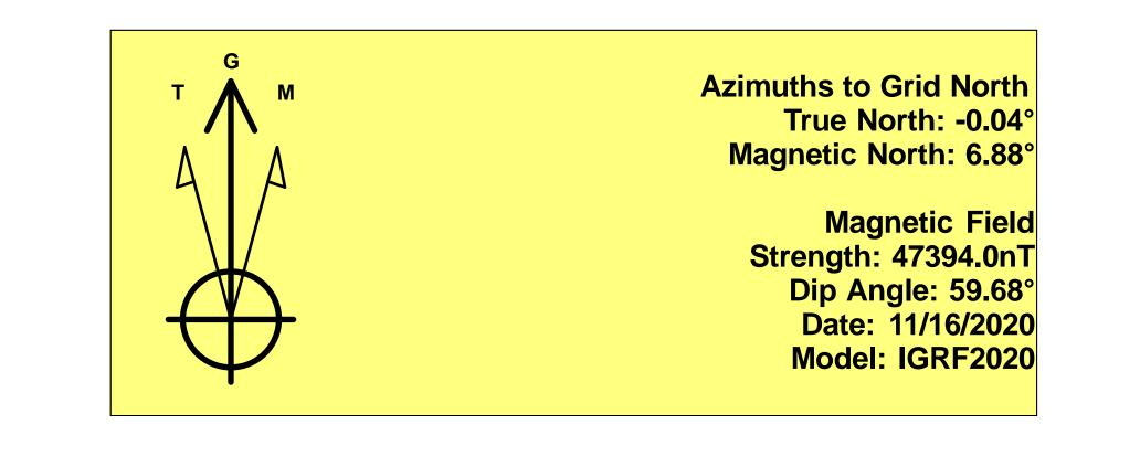
To convert a Magnetic Direction to a Grid Direction, Add 6.88° To convert a Magnetic Direction to a True Direction, Add 6.92° East To convert a True Direction to a Grid Direction, Subtract 0.04°
