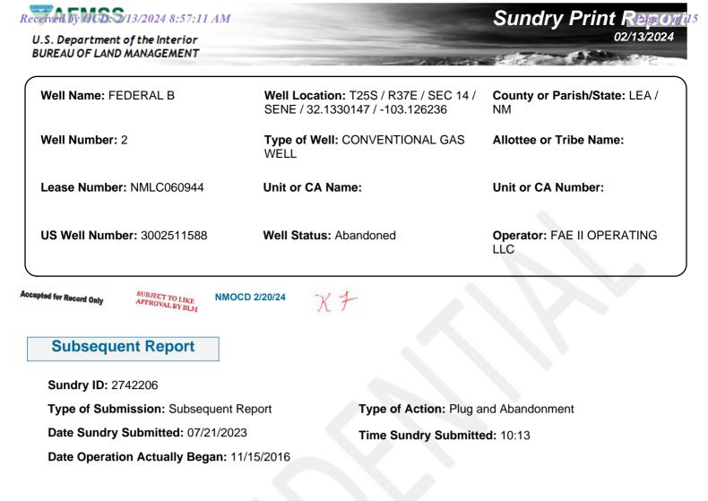
Actual Procedure: Work completed by Tora Oil & Gas LLC: Plug and Abandon Set CIBP 3100' cap w/ 25 sx cmt Queens Perf & sqz 30 sx cmt from 2280'-2150', tag. 30 sx spot from 1050'-800' top salt, tag. Perf & sqz 90 sx cmt from 350'-0' surface shoe Cut off well head Install DHM P&A completed 11/15/2016
