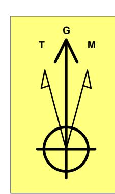
**Azimuths to Grid North** True North: -0.35° Magnetic North: 5.97°
