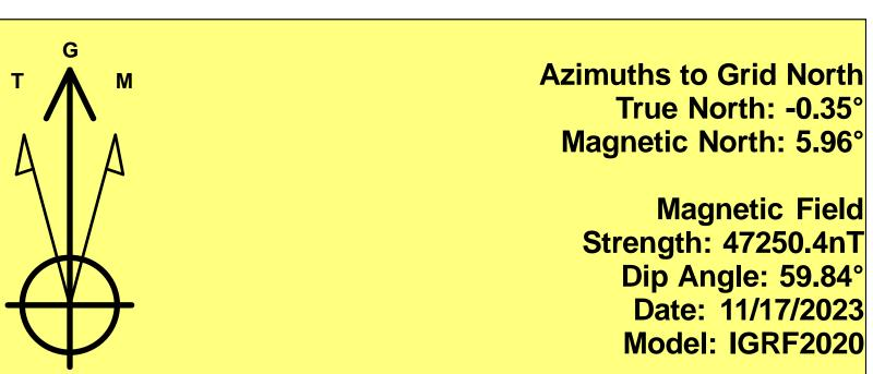
To convert a Magnetic Direction to a Grid Direction, Add 5.96° To convert a Magnetic Direction to a True Direction, Add 6.31° East To convert a True Direction to a Grid Direction, Subtract 0.35°
