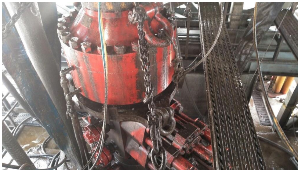
Figure 1: Winch System attached to BOP Stack
