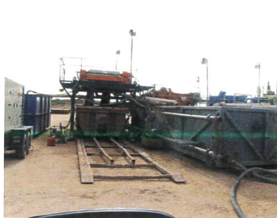
Above: Centrifugal Closed Loop System
