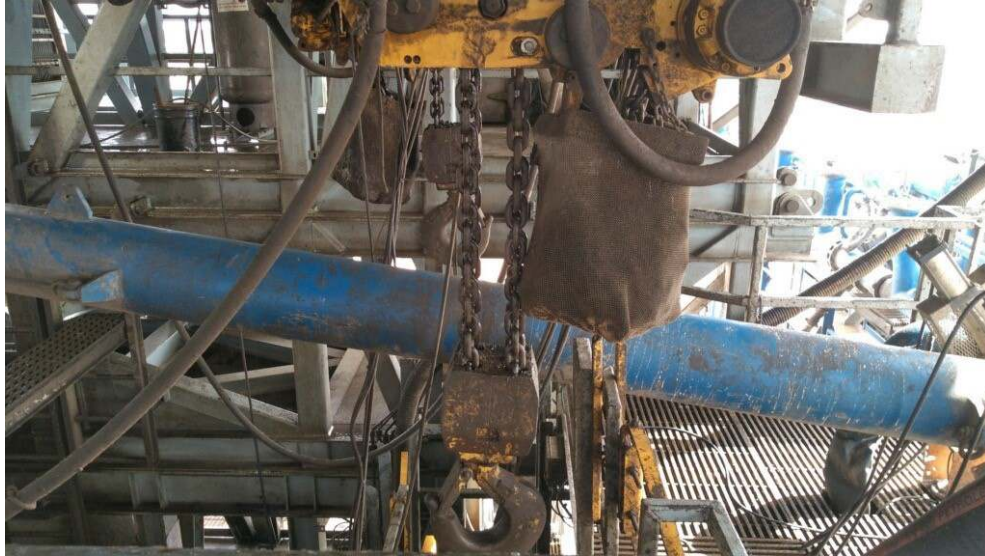
Figure 2: BOP Winch System
