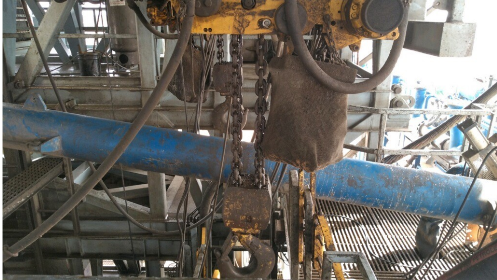
Figure 2: BOP Winch System
