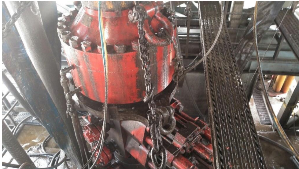
Figure 1: Winch System attached to BOP Stack
