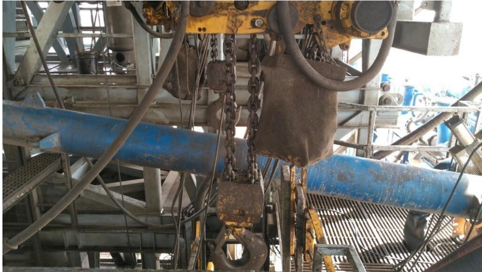
Figure 2: BOP Winch System
