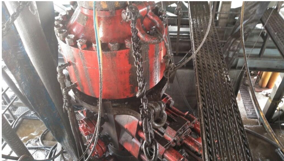
Figure 1: Winch System attached to BOP Stack
