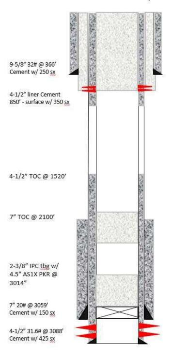
Perf through 4-1/2" and 7" at 500' and circulate 100 sacks Class C cement to surface.
