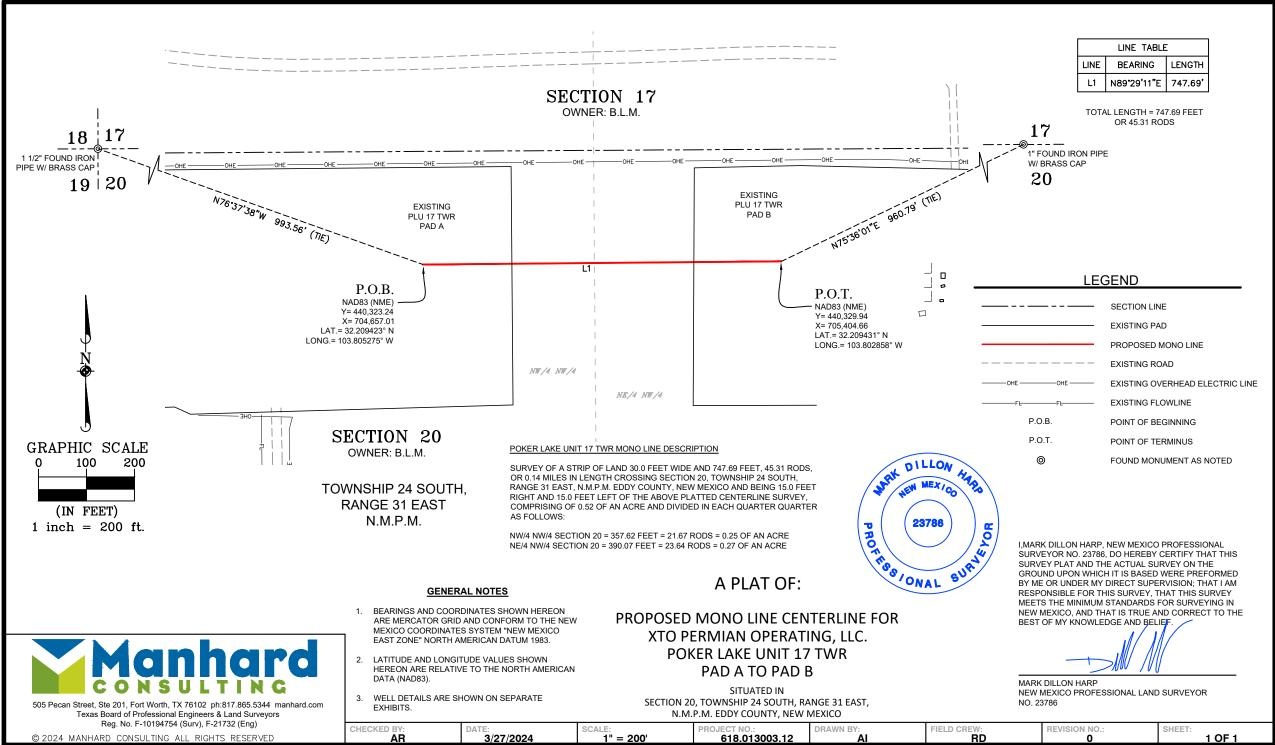
P:\618.013 XTO Energy — NM\003 Poker Lake Unit\.12 — PLU 17 TWR — EDDY\DWG\Exhibits\PAD A TO B MONO LINE.dwg
