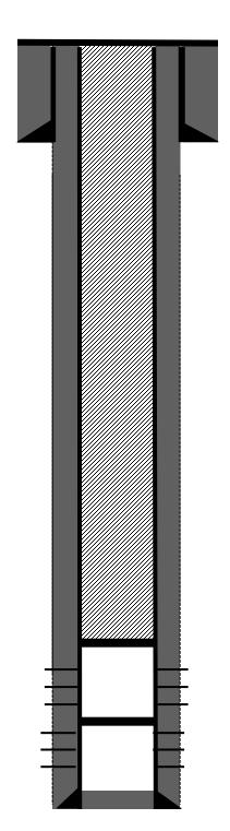
7", 20# casing @ 122'. Cemented with 70 sks Class B cement w/2% CaCl2 . Hole size: 9-7/8". Circulate 1 bbls cement to surface.
