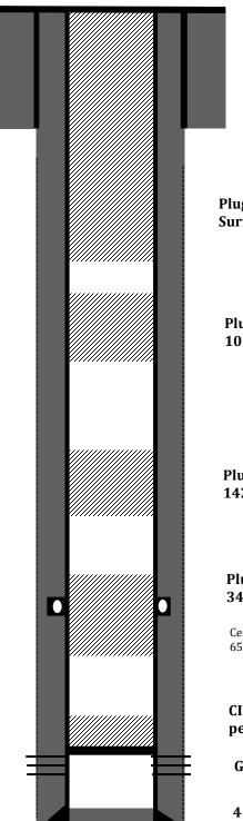
8-5/8" J-55 24# casing @ 219'. Cemented with 135 sks Class B. Circulated 2 bbls cement to surface
