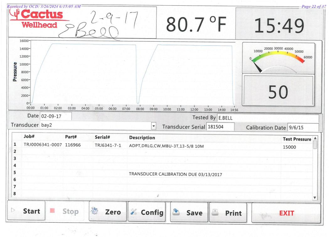
A multibowl wellhead may be used. The BOP will be tested per 43 CFR 3172 after installation on the surface casing which will cover testing requirements for a maximum of 30 days. If any seal subject to test pressure is broken the system must be tested.
