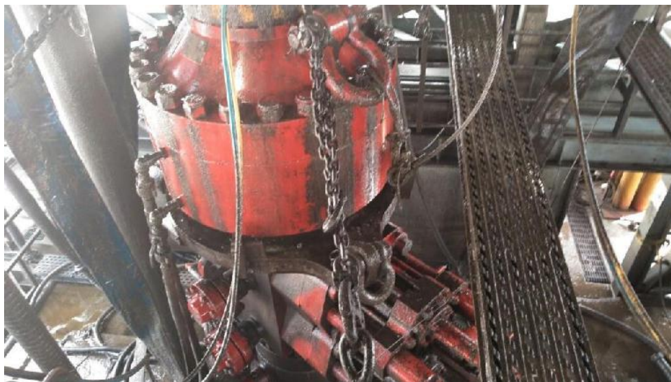
Figure 1: Winch System attached to BOP Stack
