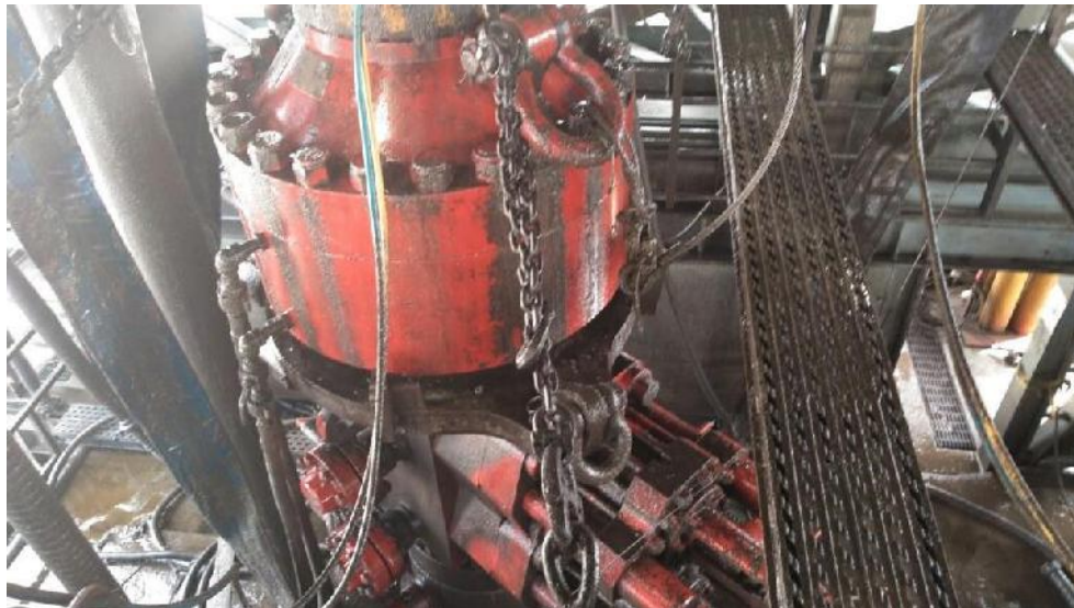
Figure 1: Winch System attached to BOP Stack
